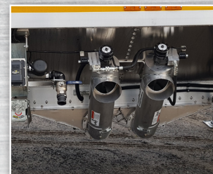
Remote Controlled and Removable Hydraulic Augers
