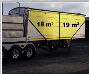
Two Dry Compartments 18m³ and 19m³ Capacities
